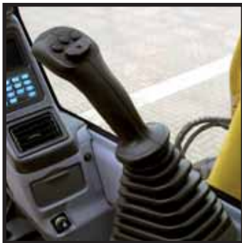
Joysticks with proportional control button for attachments
