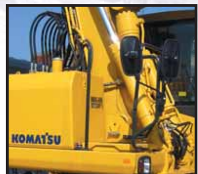
Large handrail for safe access
