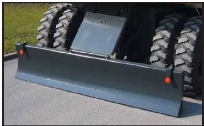
Dozer blade A parallel blade is available with standard cylinders protector for both the front and rear of the machine. Dimensions: with 2,55 m undercarriage: 2.550 mm x 520 mm with 2,75 m undercarriage: 2.750 mm x 520 mm
